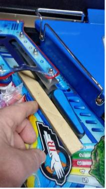
**(5)** Reinstall the flipper bats and tighten the 10mm locking nuts – **DO NOT** overtighten these nuts – they only need to be pinched up firmly. At rest, the flipper bats should align with the stainless guide rails and have about 2mm up and down movement when you have finished. Fit the included sticker under the playfield.
