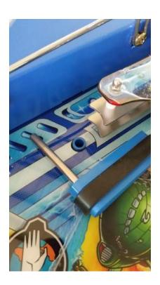
**(2)** Push fit a stainless steel sleeve supplied into each blue nylon flipper bush from the top of the playfield, initially by hand. You should be able to easily push them in more than halfway. Take care as the ends are sharp!
