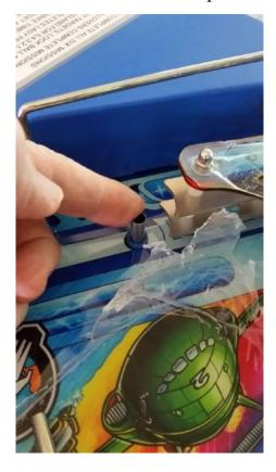
(3) With between 3 and 10mm of the new sleeve still protruding above the flush surface of the bush, apply a couple of drops of super glue between the new metal sleeve and the plastic bush.
