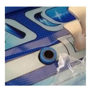
**(5)** Look carefully on the under side of the bush to see if any swarf has been pushed out of the nylon bush. If so, remove it.
