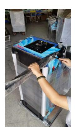
Locate the two bolts holding the machine to the steel pallet and remove these using an 18mm spanner.
