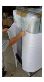
Ensure the package has no visible damage, check the 'tilt label' and don't sign for delivery if there appears to be any problems. Carefully cut the outer plastic wrap and remove the foam packing. Under the cardboard top packing you will find the setup instructions as well as the service manual.
