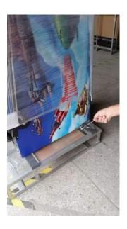
Now tip the machine onto the front legs. Raise the back and sit it on a stool or similar so that the back legs can be bolted on.
