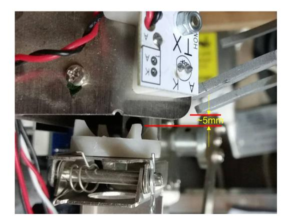
The mounting position of the wireform at the ball entry end is not critical.
