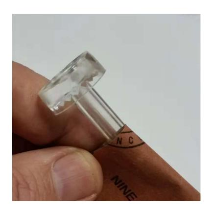
(4) Refit the button and "C" clip and check for smooth operation. Refit the LED PCB.
