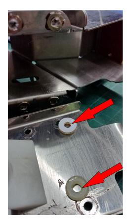
(8) Fit the replacement front plate with the four screws and two locknuts and re-fit the mech to the playfield.
