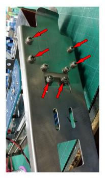
(7) remove the front plate and if your mech has two x 2mm plastic spacer washers fitted with the top two screws, discard these (no longer required) as well as the old front plate.
