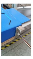
(3) Remove the four screws holding the "ball trap" mechanism cover in place and remove the cover and the railway train inside (the base can stay in place).
