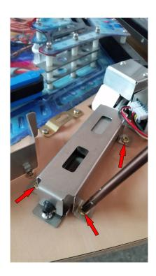
(4) remove the three screws that secure the coil and its frame to the main trough mechanism and carefully allow the coil to hang by the wires.
