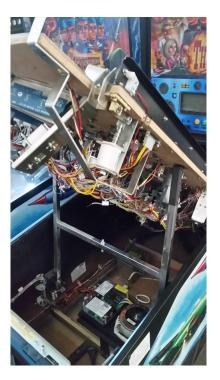
(3) Remove the three screws holding each bracket to the playfield.
